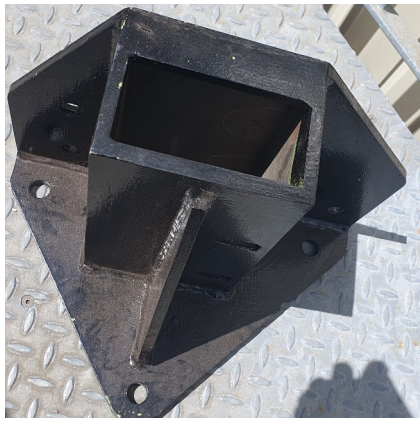
BR Mk1 Vestibule Buffer Stem Bracket. Steel fabrication.
